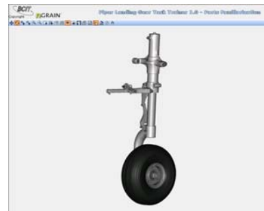
Virtual task trainer of Piper landing gear
